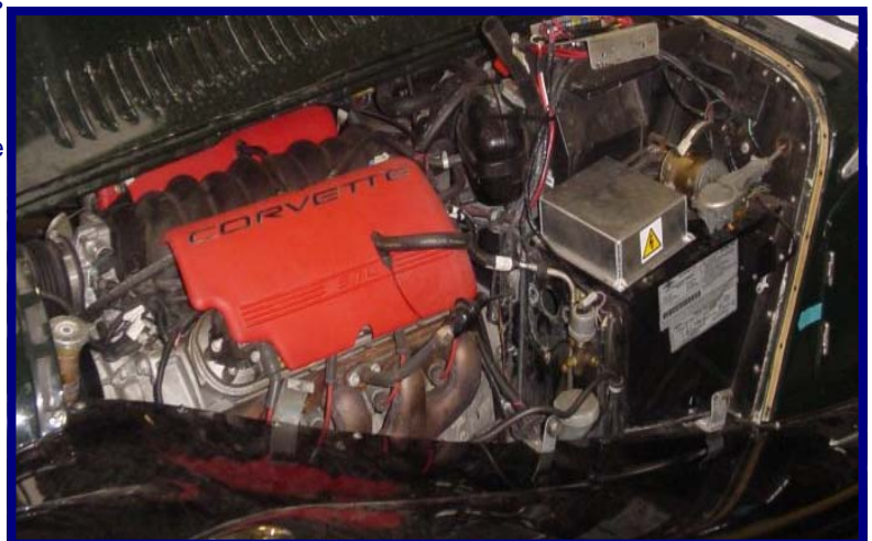
5.7L V 8 Corvette powered Classic Morgan with EPAS steering
